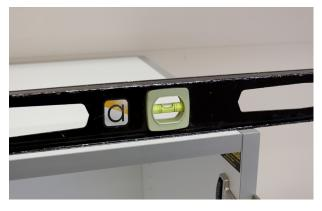
7. Continue to adjust each of the levelers until the cabinet is level side to side, and front to back.
