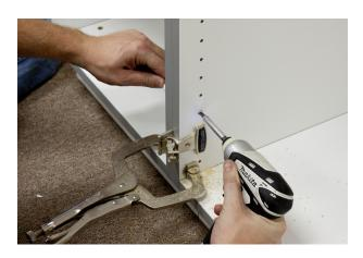
20. Use the provided connecting bolts in the hardware box to secure the top and bottom of the side panels together.
