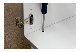
6. Level this cabinet by accessing levelers through the holes in the cabinet floor. Use a 4 mm Allen wrench to adjust the height of each leveler as needed.
