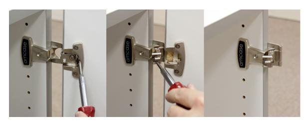
5. Remove all the doors from the overhead cabinets before installing them. Using a Flathead screwdriver, release the hinge from the door mount. A slight turn may help to release it.
