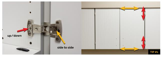
5. Remove the hinge cover cap and turn the adjustment screw. This adjusts the door up and down. The adjustment screw in the door mount adjusts the door side to side.
