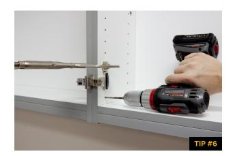
13. Using a 1/4" drill bit, ream one system hole on the top and one on the bottom of the side panels for connecting bolts.
